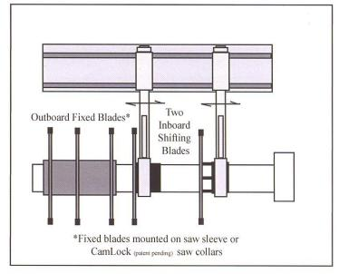
Inboard shifting saws allow quick access of fixed saw blades providing the industry's fastest change-overs.
