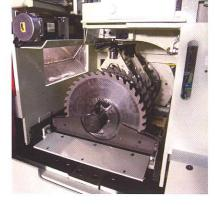
Heavy-duty overbeam provides an extremely rigid support for the shifting saw carriages.
