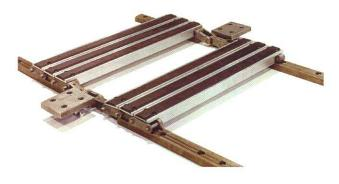
High friction "Posi-Feed" bed featuring aluminum slats with replaceable steel-backed rubber inserts. Precision feed chains ride on hardened steel "Double-Vee" rails.
