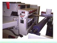
Optional machine mounted Power Table for automatic feeding provides improved accuracy and reduces operator fatigue.
