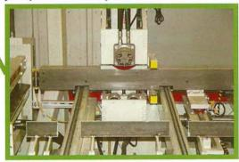
Accumulator arms with integrated board dealer allow a single operator to control the system
