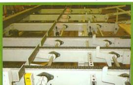
System guide is mounted on linear ways for smooth and accurate positioning integrated with Rip Navigator control. Integral upper and lower rolls both jump for accuracy and reduced wear
