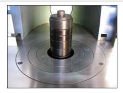
THE THREE INCLUDED TABLE inserts allow for various cutter diameters.
