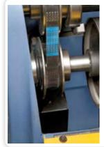
TRADITIONAL VARIABLE SPEED pulley system eliminates the troubles prone to frequency drives.
