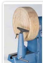
THE INCLUDED OUTBOARD SUPPORT and tool rest allows a huge 35" swing over the bed.
