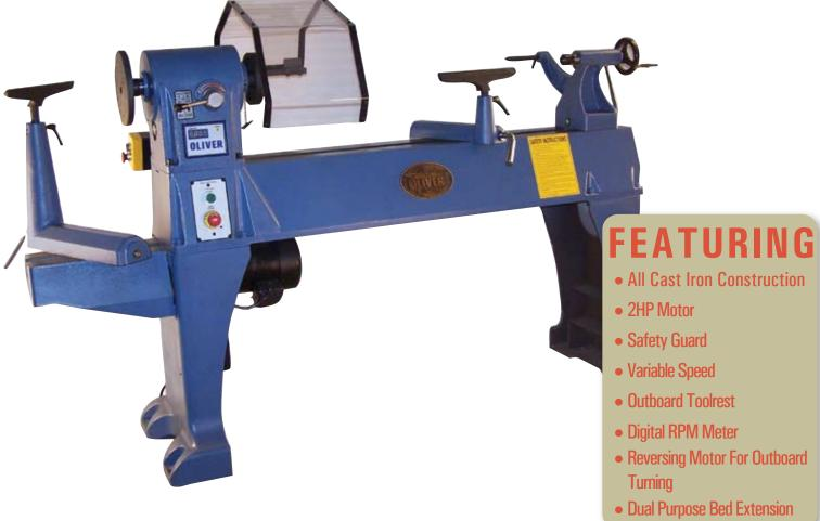
The Oliver 2018 Classic Lathe brings the Lathe back to the Oliver Line, and in true Oliver fashion. Starting with an all inclusive cast iron construction for torsional rigidity. Next, Oliver adds a reversible 2HP motor with a wide speed range for a variety of tasks. In addition, an RPM meter displays an accurate turning rate
