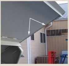
Sides of hopper extend down past hopper bottom for added strength
