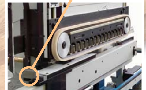
Work-piece feed system and upper-pressure system with detail of back-up blocks.
