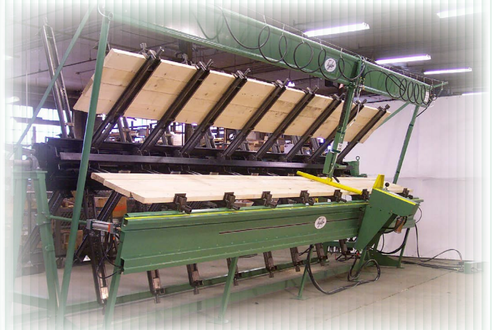
Custom Shop Clamp Carrier For Long Stock - 16' Rail & Posts
