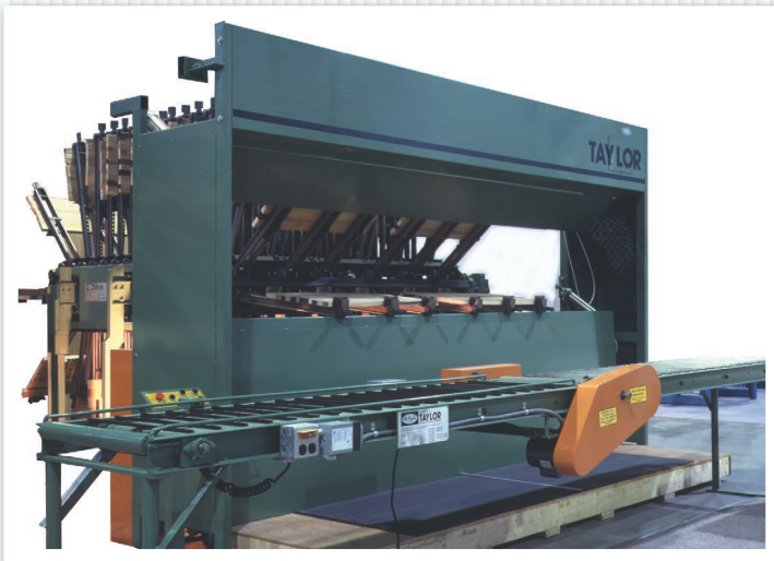
Dual Automated Clamp Carrier circa 1990
