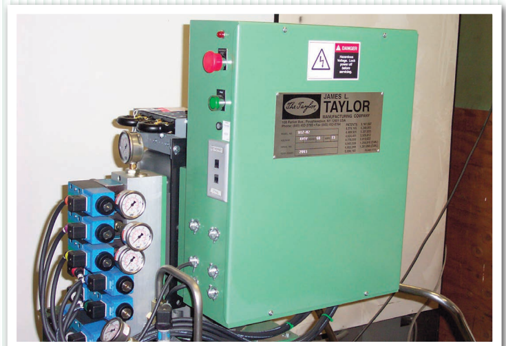
"Smart Clamp" Connected to Ethernet
