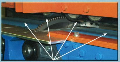
The new Duo-Drive<sup>™</sup> is the only saw in the world to have the patented top and bottom belt drive system.
