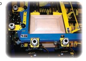
Produce up to 100+ Miter Cabinet doors per day. JLT Door Clamps ship Pre-assembled for a quick and easy installation.
